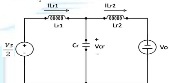
Fig. 6. Equivalent circuit for Mode I.
