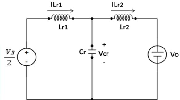
Fig. 4. Equivalent circuit for the proposed converter
