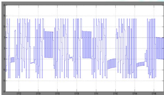
Fig. 13. Voltage out from resonant tank
