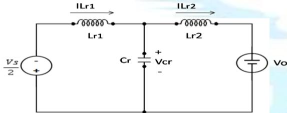
Fig. 8. Equivalent circuit for Mode III.
