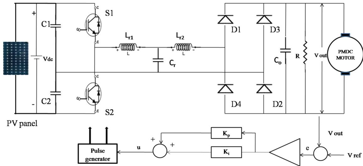
Fig.3. Circuit diagram for solar resonant converter fed PMDC motor
