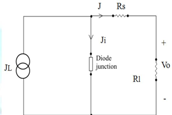
Fig. 1. Equivalent circuit of PV cell
