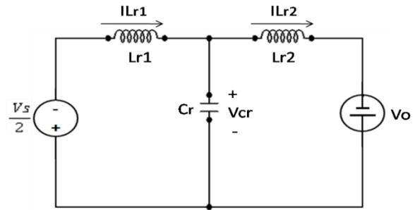
Fig. 9. Equivalent circuit for Mode IV
